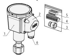
Radial density monitor with PA injection molding electrical connector housing
