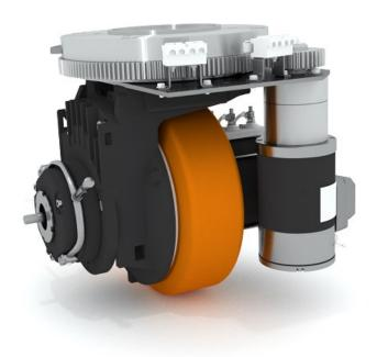
The motor-in-wheel drive unit (MIWD) is an ideal choice for almost any indoor electric vehicle with a wheel load up to 3200kg. The compact design minimizes the space needed for the installation. All components except for cables and wires are located under the vehicle body, freeing up much needed space inside the vehicle.
