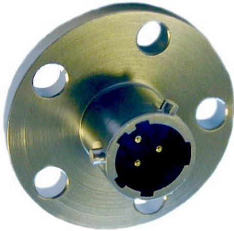
6100 is a very robust stainless steel flange connector, designed for heavy duty use in hydraulic applications. Mostly as a hydraulic pressure sealing on the cylinder wall, keeping the oil inside but electrically connecting the incorporated sensor with the system outside.
